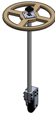
Figure 3: SolidWorks rendering of the hand steering module
